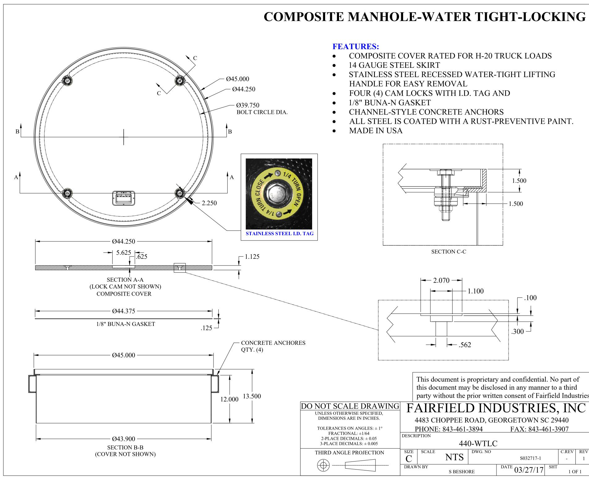
COMPOSITE COVER RATED FOR H-20 TRUCK LOADS STAINLESS STEEL RECESSED WATER-TIGHT LIFTING ALL STEEL IS COATED WITH A RUST-PREVENTIVE PAINT.
